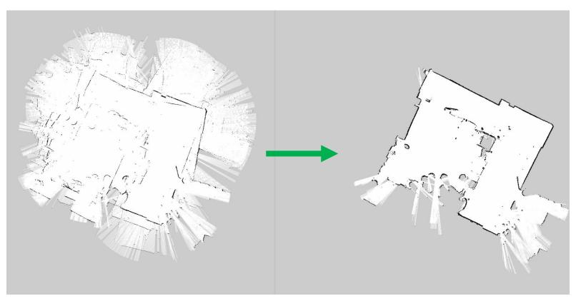
Mapping integrates sensor readings (e.g., laser range scanner) together reducing odometry error thus obtaining a valid map of the environment
