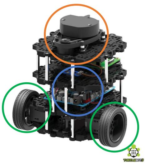
For example, one node controls a laser range-finder, one Node controls the robot's wheels motors, one node performs mapping, one localization, one node performs path planning, one node gives velocity commands to the wheels, one node provides a graphical view of the system, and so on.
