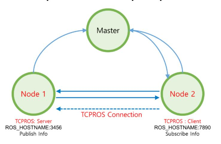
At this point a direct connection between publisher and subscriber node is established using TCPROS (TCP/IP based protocol)
